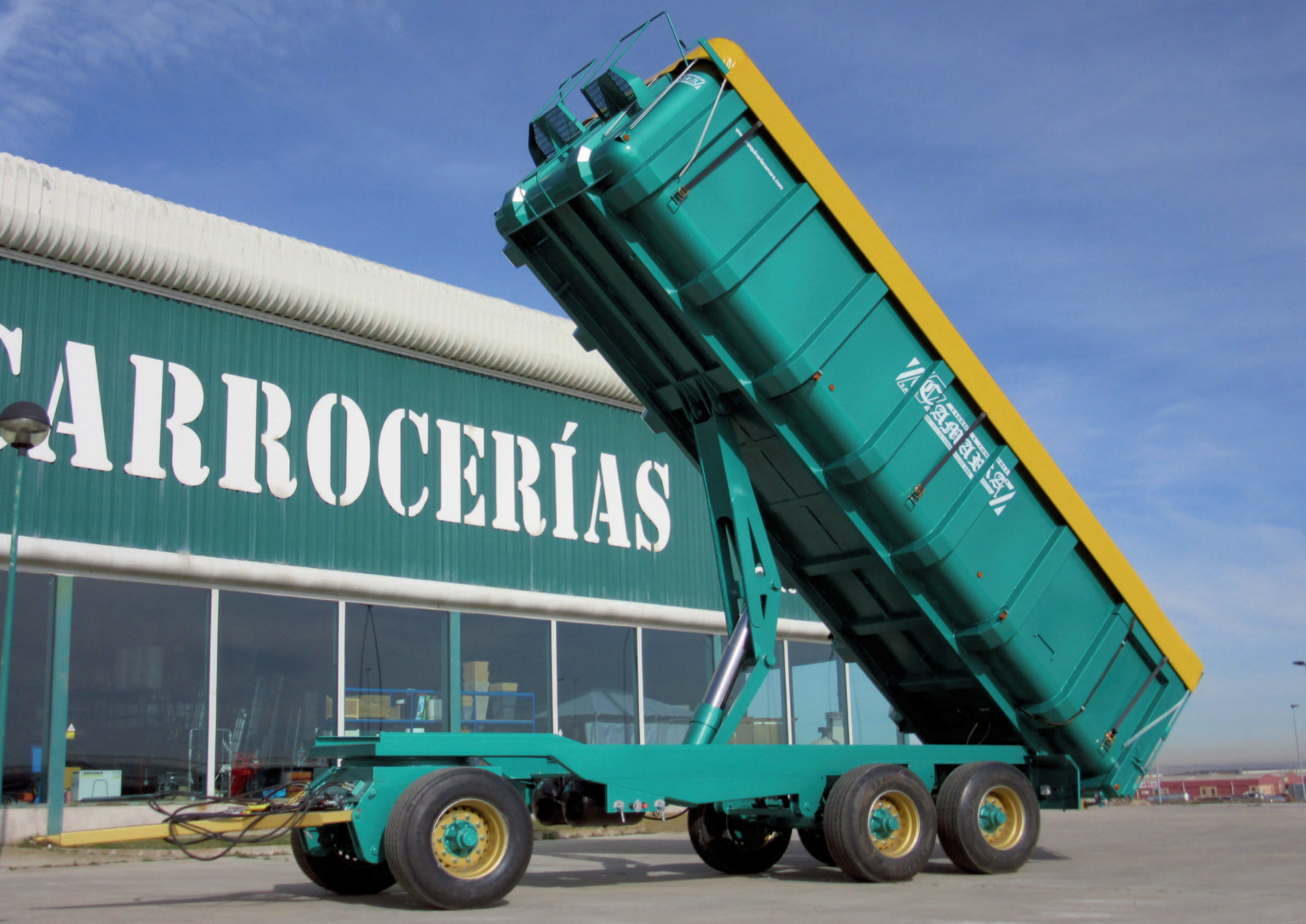
Puerta hidráulica y automática Door with double opening feature: hydraulic and automatic. Porte hydraulique et automatique
