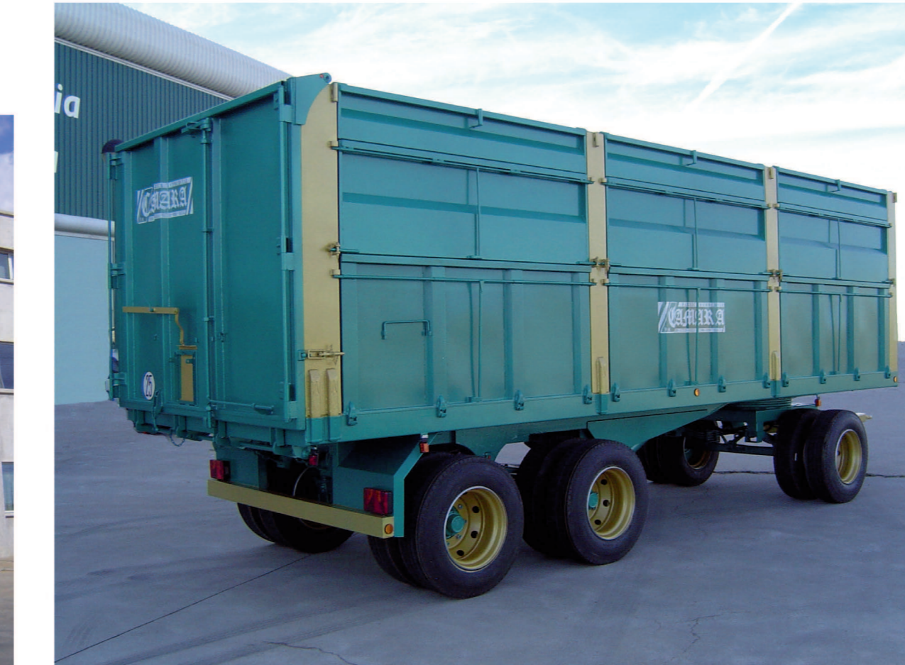
Apertura de 2 hojas sin travesaño Opening for the 2-leaf door with absent crossbar. Ouverture de 2 vantaux sans traverses
